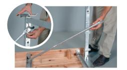
The Leg Frame Brace fits into a slot on the underside of the dock and is secured to the dock leg pin with a hairpin cotter key.
